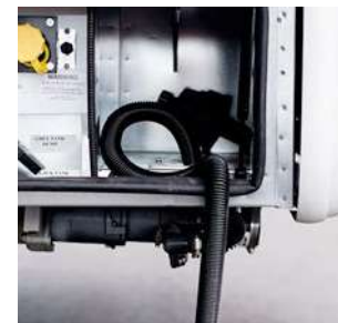
Macerator Sewage Discharge c/w Manual Disconnect
